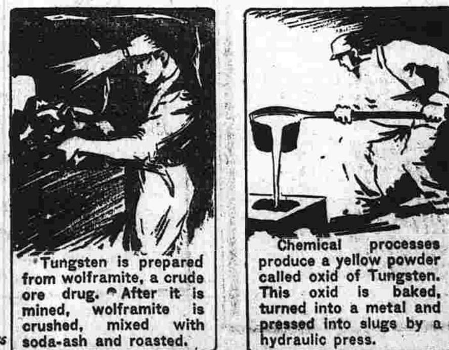
Tungsten is prepared from wolframite, a crude ore. After it is mined, wolframite is crushed, mixed with soda-ash and roasted.
